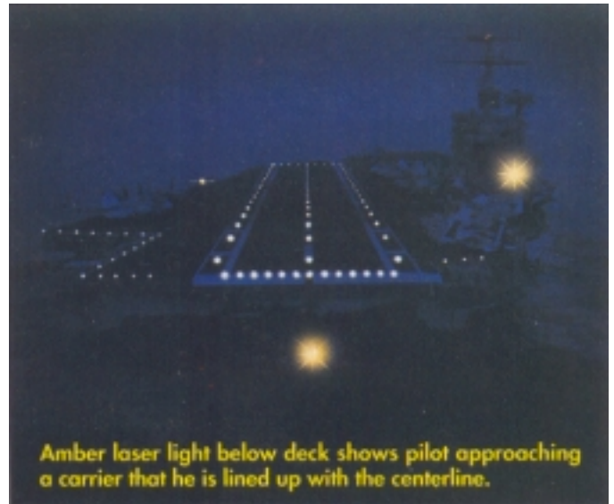
Laser Centerline Localizer, stabilized by electric actuators to compensate for roll and pitch of the carrier, has six amber lights flanked by green and red.
